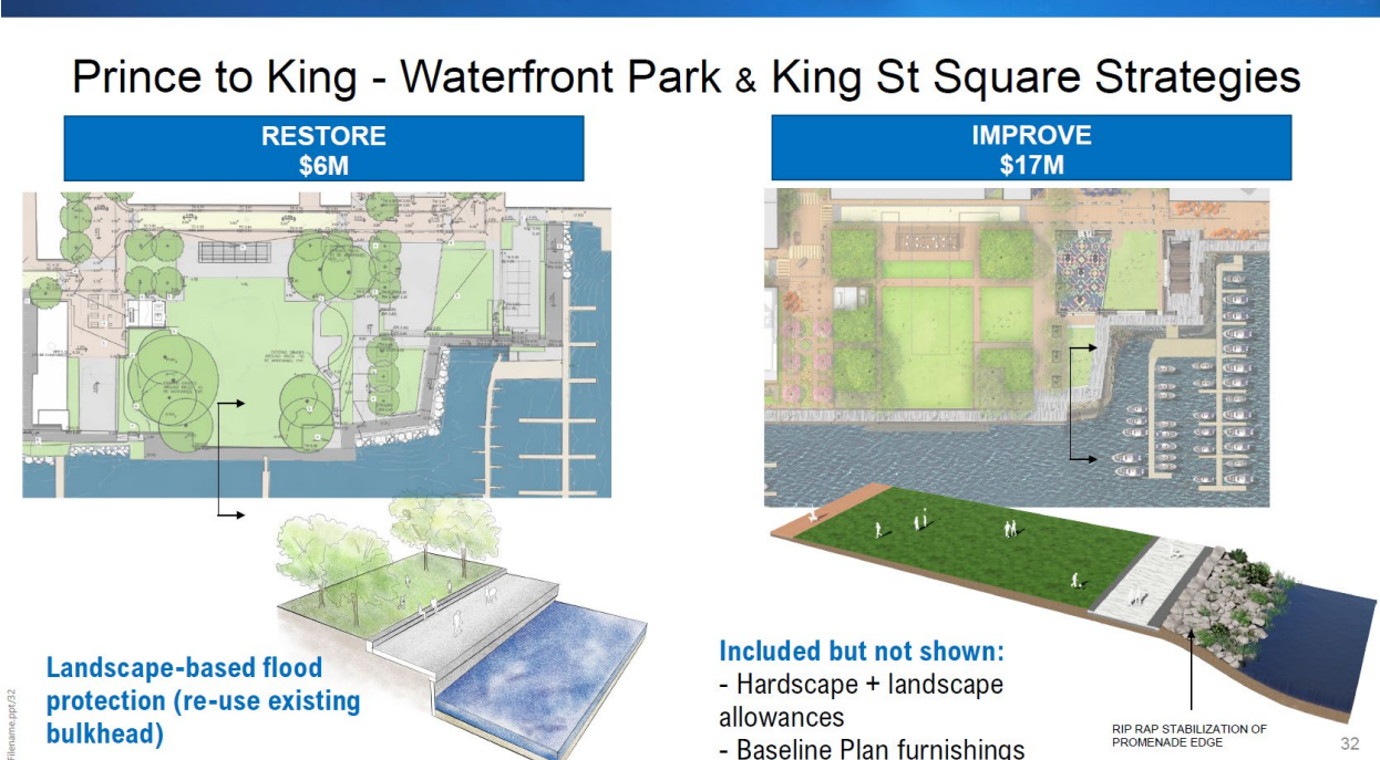
126 127 Figure 3: Landscape-Based Flood Protection at Waterfront Park
